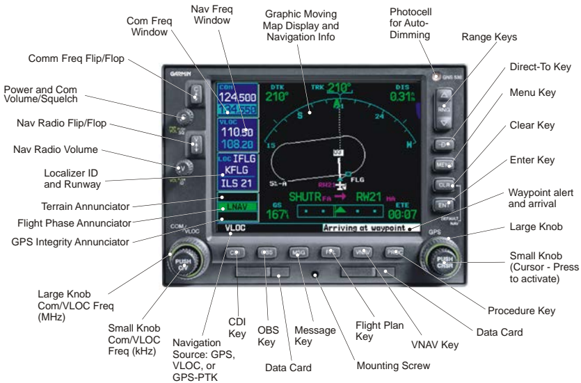
Figure 1 - 530W Series Control and Display Layout
